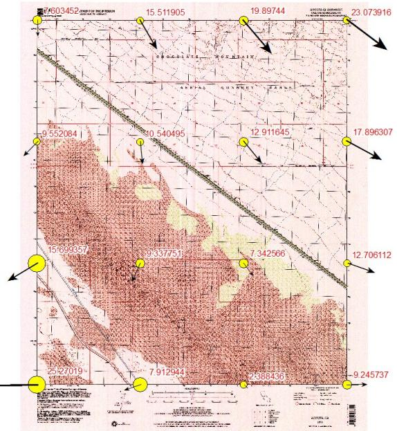
Fig. 2: Residual error vectors (direction and magnitude) for the GCPs used for georeferencing the maps obtained by least squares second order polynomial transformation.
