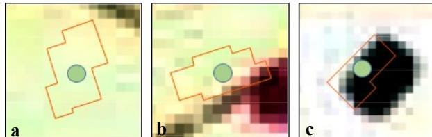
Fig. 1: Examples of positional offsets between building symbols and contextual data: (a) significant offset (map symbol outside the subimage), (b) moderate offset (partial overlap) and (c) minor offset (mostly overlapping)
