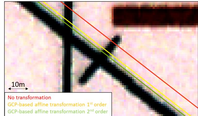
Fig. 3: Effect of the alignment of contextual data to map distortions introduced by GCP inaccuracies shown for a railroad on a USGS topographic map.
