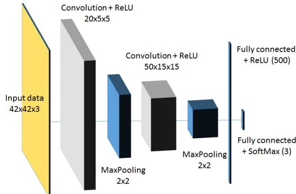
Fig. 8: Layer configuration of the LeNet CNN applied.
